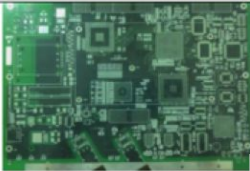
Solder Mask With Copper
