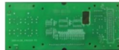
Solder Mask With No Copper
